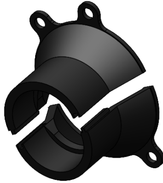
Figure 11: Bearing casing interface with rear PPAE exploded view
