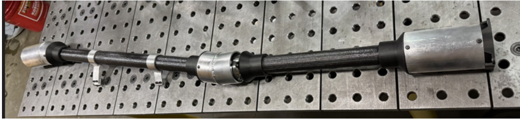
Figure 4: 4WD guarding on propshaft prior to first drive
